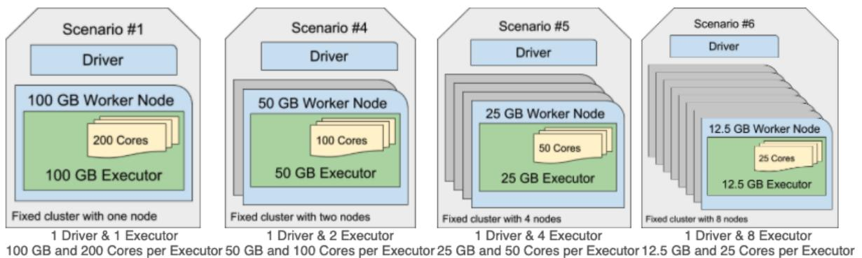
Note: each configuration has roughly the same compute power using 100GB of RAM and 200 cores.
